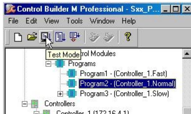
7. Click the “Continue” button for the On Line Change analysis dialog and observe that Control Builder enters the “Test” mode
